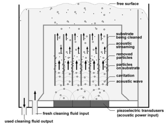
**Fig. 6. Schematic of USC/MSC tank and the physical phenomena induced by the piezoelectric transducers [4].**
