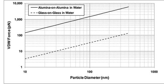
**Fig. 3. Plot of VDW force versus particle in water medium.**
