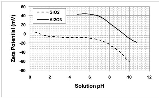
**Fig. 5. Plot of zeta potential of alumina and silica as function of solution pH [7].**
