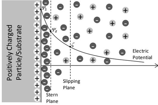
**Fig. 4. Schematic of the electric potential variation in a liquid medium in the proximity of a solid object.**
