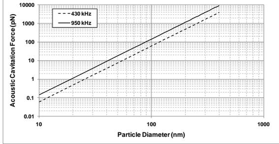
**Fig. 14. Plot of acoustic cavitation force versus particle diameter for two different transducers frequencies: 430 kHz and 950 kHz.**
