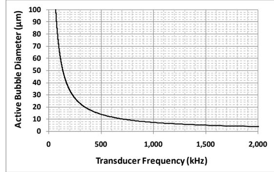
**Fig. 12. Plot of active bubble diameter versus transducer frequency.**
