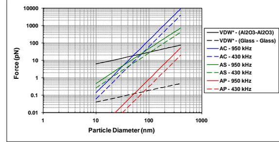
**Fig. 15. Plot of detachment forces and scaled VDW forces for the cases of alumina-on-alumina and glass-on-glass.**
