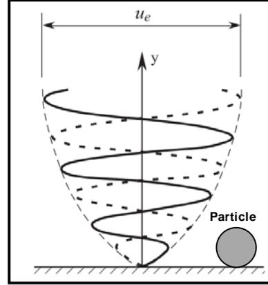
**Fig. 8. Schematic of the velocity profile within an acoustic boundary layer that a particle experiences. The sketch shows the velocity profile at two instants separated by one-half period [11].**
