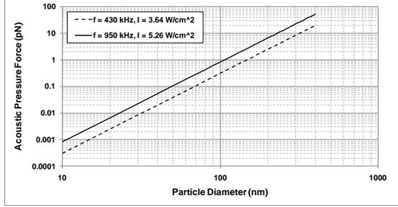
**Fig. 11. Plot of acoustic pressure force versus particle diameter for two different transducers: a) a transducer with  $f = 430$  kHz,  $I = 3.64$  W/cm<sup>2</sup>; and, b) a transducer with  $f = 950$  kHz,  $I = 5.26$  W/cm<sup>2</sup>.**
