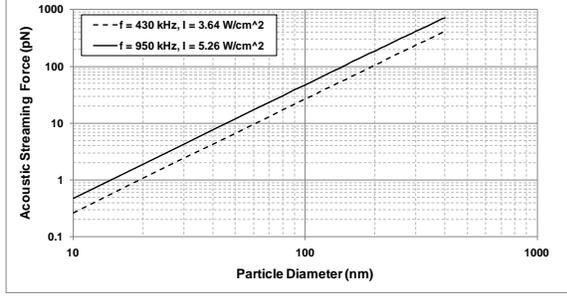
**Fig. 9. Plot of acoustic streaming force versus particle diameter for two different transducers: a) a transducer with  $f = 430$  kHz,  $I = 3.64$  W/cm<sup>2</sup>; and, b) a transducer with  $f = 950$  kHz,  $I = 5.26$  W/cm<sup>2</sup>.**
