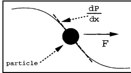
**Fig. 10. Schematic of a pressure variation wave induced by an oscillating transducer (top) and the pressure gradient across a particle (bottom) [13].**
