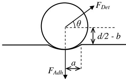
**Fig. 2. Diagram of equivalent adhesion and detachment forces acting on a spherical particle that is attached to a substrate.**
