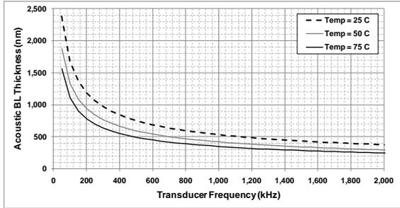
**Fig. 7. Plot of acoustic boundary layer thickness versus transducer frequency for various solution temperatures.**
