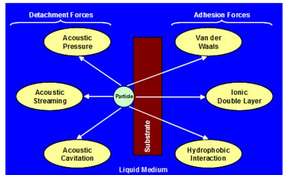
**Fig. 1. Schematic of adhesion and detachment forces acting on a particle attached to a substrate in a liquid medium.**
